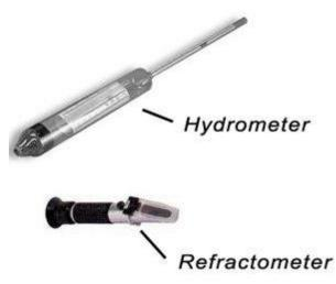
buoyed up by a force equal to the weight of the liquid displaced. Thus, the lower the density of the solution, the lower the Hydrometer will sit [1].
